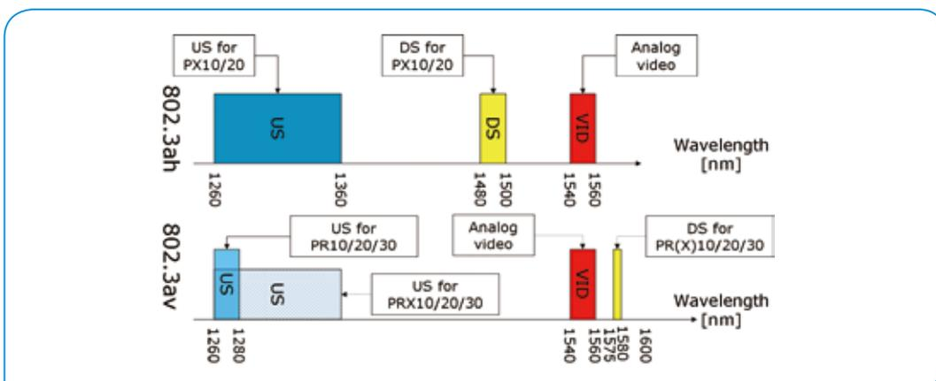
Figure 4 10G EPON Wavelength Allocation Chart
